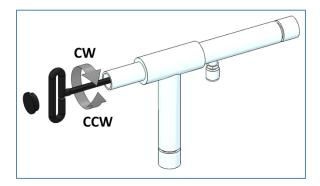
To increase the pressure setting, rotate clockwise.
