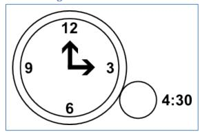
Bulb placement should be at the 4:30 position of a clock on the suction line.
