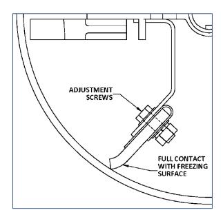
With normal usage, the Squeegee can wear over time. Worn Squeegees need to be trimmed or replaced.
