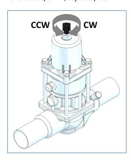
To increase the pressure setting, rotate clockwise.
