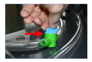
Open Ice Flaker Stop Valve to allow water to exit from Water Sump.
