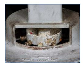
The effects of scale and sediment can be very destructive to the Ice Flaker.
