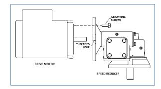
Drive Motors may provide a good deal of resistance when being removed. There are (2) threaded holes on the face of the Speed Reducer in which the mounting screws can be inserted to help push the Drive Motor away.
