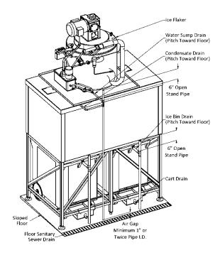
The Drain Water Piping figure above illustrates the recommended piping to a floor sanitary sewer hub or trench drain. The two vertical pipe drops should drain water through an indirect water connection with an "Air Gap". Code authorities having jurisdiction may dictate other indirect water connection requirements.
