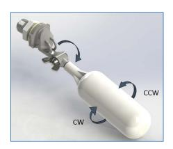
Adjust the water level by loostening the wing nut then raise or lower the arm to make adjustments to desired water level. Tighten wing nut, test for proper level and adjust again if necessary.
