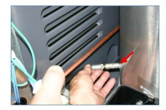
Over-greasing may "pop" the seal out of its normal position.
